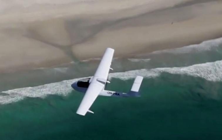
The Eagle Eye I is our amphibious aeroplane from Technokontrol to be used as an efficient aerial observation and safety control platform. It has a two seats side by side assembly with a large cockpit (1.10 m width) and with exceptional visibility.
