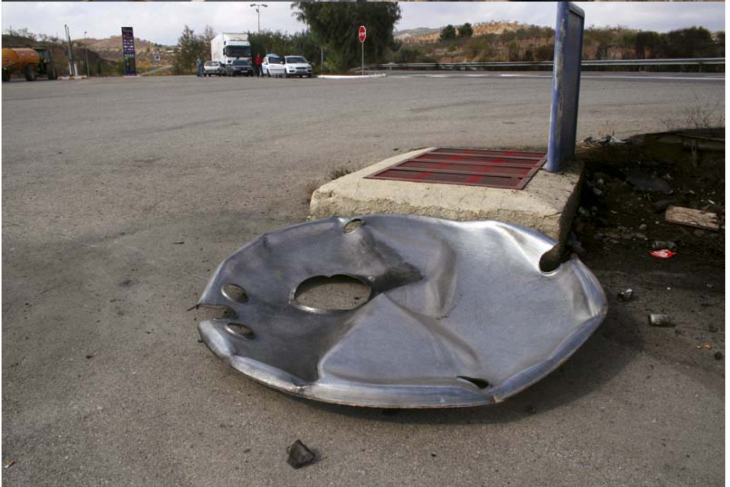
Figure 13. In the foreground, two of the baffle plates of the road tanker. Source: On-the-spot witness.
