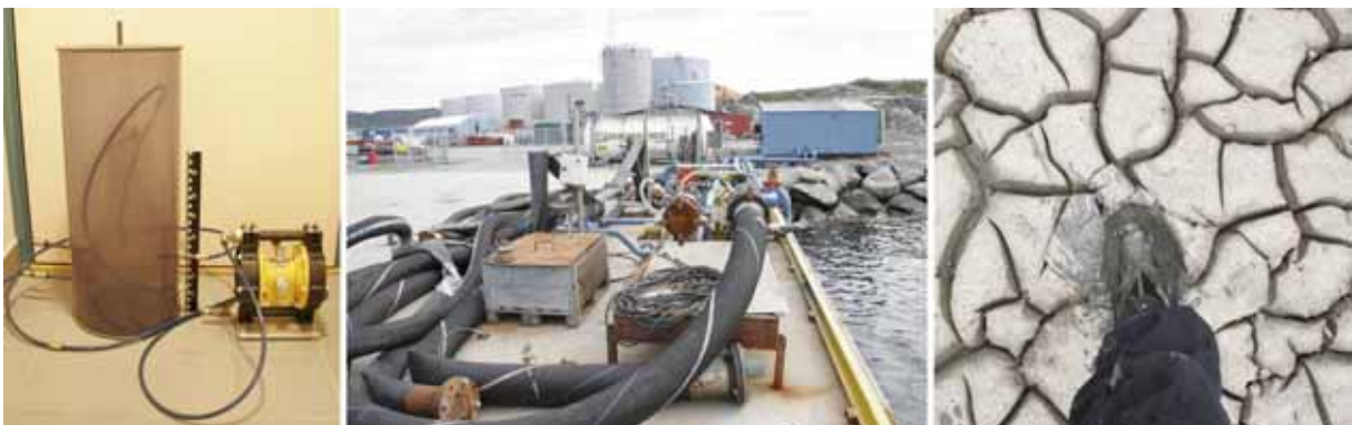
Figure 1-3 The small-scale apparatus used to investigate the effect of adding hydrochloric acid solution to the solid waste (left); the tank facility seen from the quay, with the lye tank ('De Rijke'), and the flexible tubes used for transferring coker gasoline from the tanker to the tanks (centre); the remaining substance on the ground inside Tank Farm II after the accident (right); pictures provided by the Norwegian Police.
