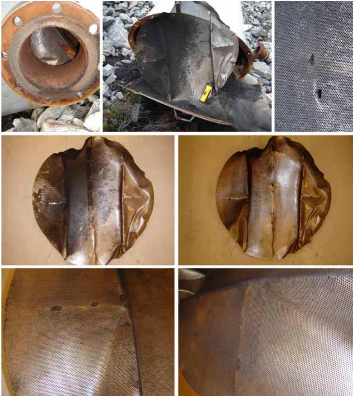
Figure 6-5 The perforated stainless steel plate from the bottom of the air filter: the plate viewed through the inlet to the canister (upper left); the plate removed from the canister, with a deposit of soot covering about half the surface area (upper centre); holes in the plate at old spot welds, presumably formed during deformation of the plate upon impact of the canister (upper right); the plate before (left middle) and after (right middle) removing the soot deposit; discolouration of the surface of the stainless steel plate, characteristic of heat tinting (lower left and lower right). Photos by T. Skjold.
