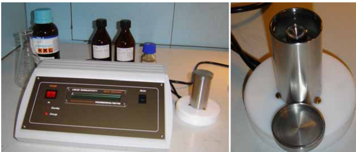
Figure 6-1 The liquid conductivity meter, Model L40 from Wolfson Electrostatics, with the bottle of calibration fluid ( n -heptane) and 3 samples of alkaline waste (left); close-up of the measuring cell (right).
