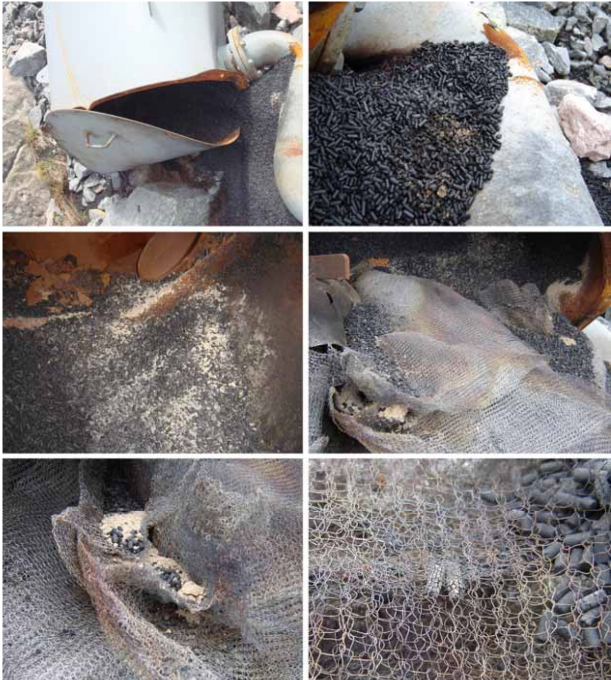
Figure 6-6 Filter medium, ash like material, and stainless steel wire fabric from the air filter: activated carbon granules poured from the canister, with a pinch of ash-like material (upper left – photo taken by Ø. Larsen during the first on-site inspection on 31 st May 2007). Close-up of the ash-like material beside the canister (upper right); activated carbon granules with ash like material near the inlet to the canister (middle left); stainless steel wire fabric with evident discolouration (middle right); close-up of stainless steel wire fabric with whitish ash like material (lower left); close-up of activated carbon granules between layers of stainless steel wire fabric (lower right); photos taken by T. Skjold during the second on-site inspection on 18 th July 2007.
